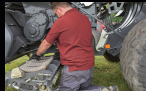
Ample accessibility offering straightforward knife removal
